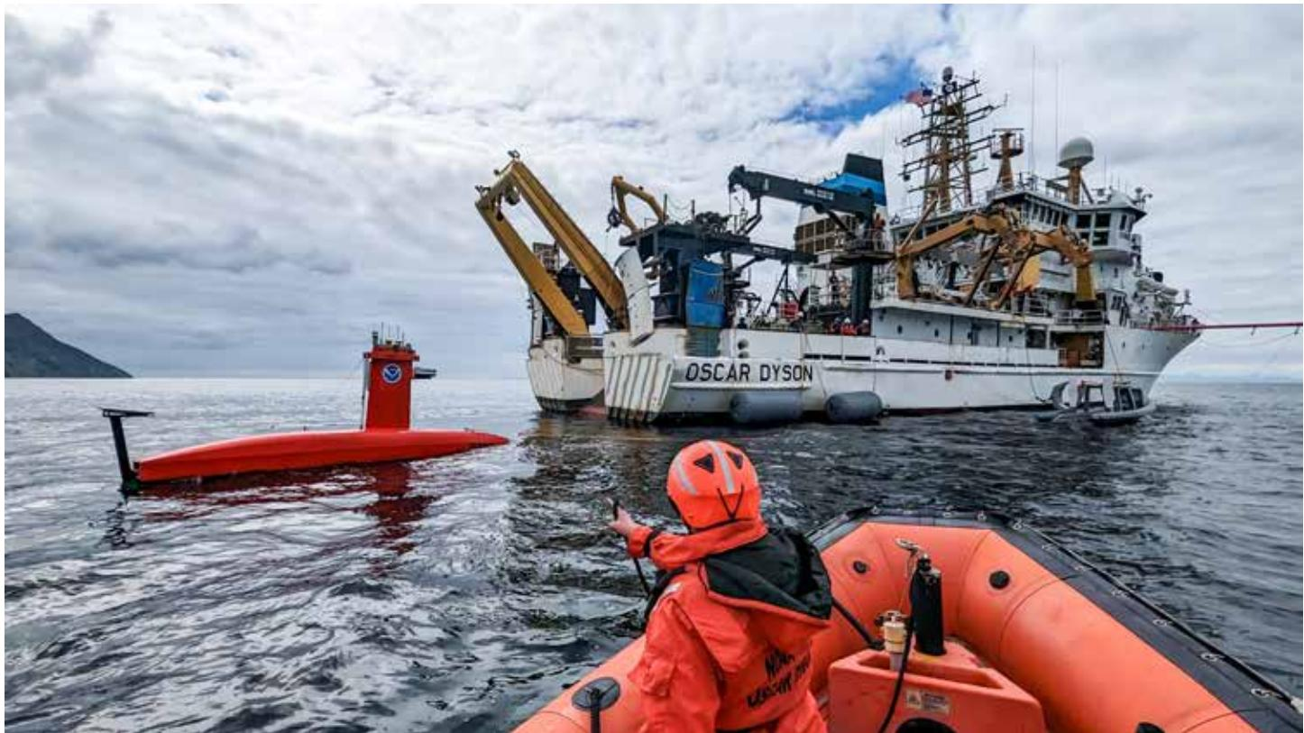
NOAA is expanding its use of uncrewed systems to collect data on the ocean and atmosphere, and NOAA Corps officers are playing a leading role in that effort. Here, a small boat crew follows NOAA's DriX uncrewed surface vehicle during a test launch from NOAA Ship Oscar Dyson off the coast of Alaska. Photo: Lt. Cmdr. Bryan Begun, NOAA Corps
