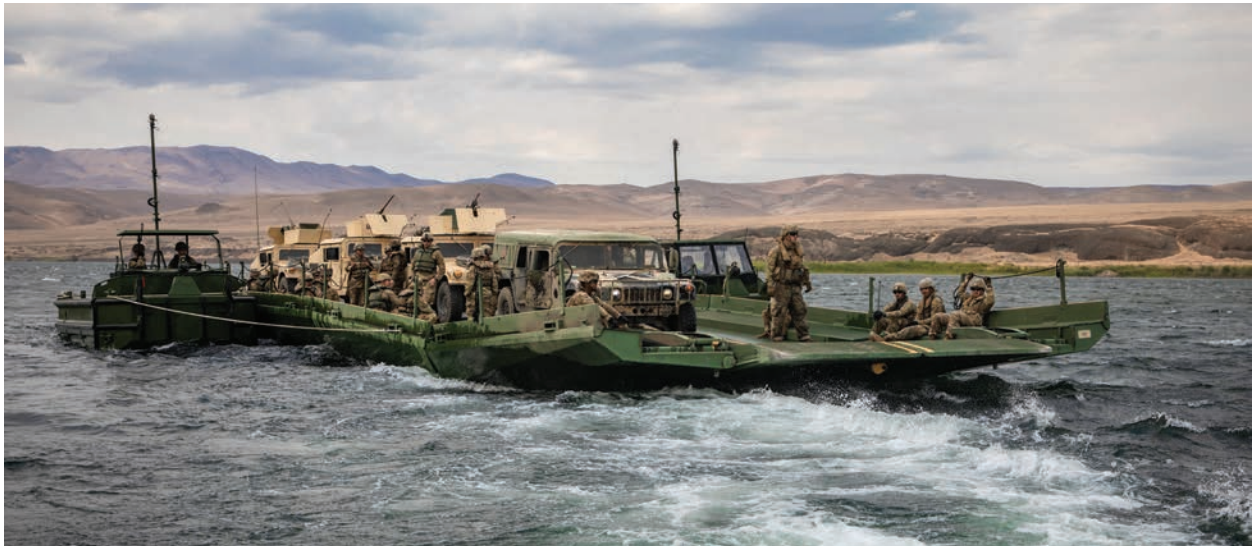
Engineers with the 671st Engineer Company and 301st Maneuver Enhancement Brigade cross the Columbia River aboard an Improved Ribbon Bridge (IRB) raft system at the Yakima Strike exercise, Washington, August 17, 2021. (Photo by Sgt. John Weaver)
