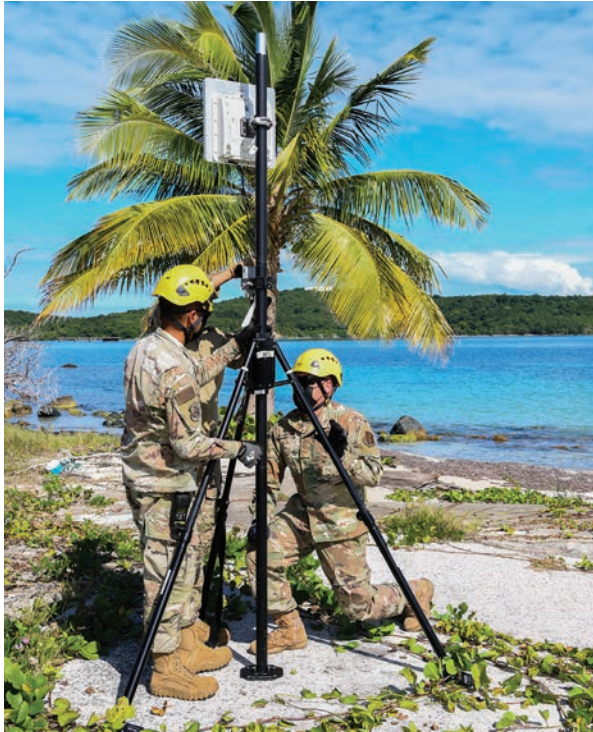
U.S. Airmen with the 156th Communications Flight, Puerto Rico Air National Guard, assemble a point-to-point microwave to receive network capabilities from the Joint Incident Site Communications Capability to their alternate location during training at the Roosevelt Roads U.S. Army Reserve Center in Ceiba, Puerto Rico, Dec. 9, 2020. Airmen with the 156th CF are conducting training with new team members on updated JISCC equipment. (U.S. Air National Guard photo by Master Sgt. Caycee Watson)
