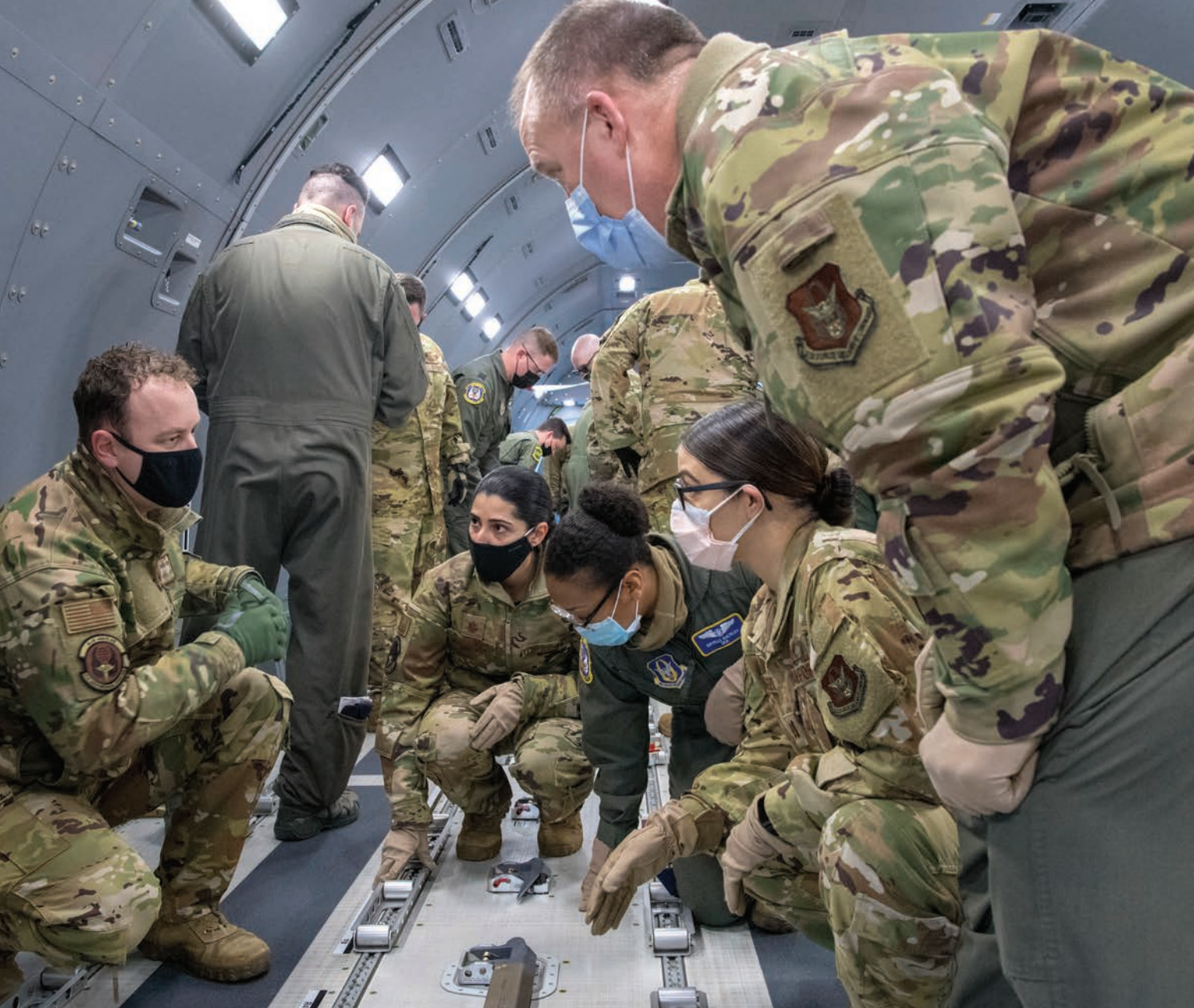
Master Sgt. Ryan T. Wood, a Air Mobility Command Headquarters command aeromedical evacuation training manager assigned to Scott Air Force Base, Ill., instructs members of the 514th Aeromedical Evacuation Squadron on how to remove rolling tracks from the floor of a KC-46 Pegasus Feb. 26. Members of the 514th AES flew a training mission to Isla Verde, Puerto Rico, with Air Force Reserve Command, Air Mobility Command, and the 916th Air Refueling Wing, Feb. 26, 2021. Members from the 514th AES were evaluated on many different scenarios designed to replicate real-world combat medical service in flight. (U.S. Air Force photo by Senior Airman Ruben Rios)
